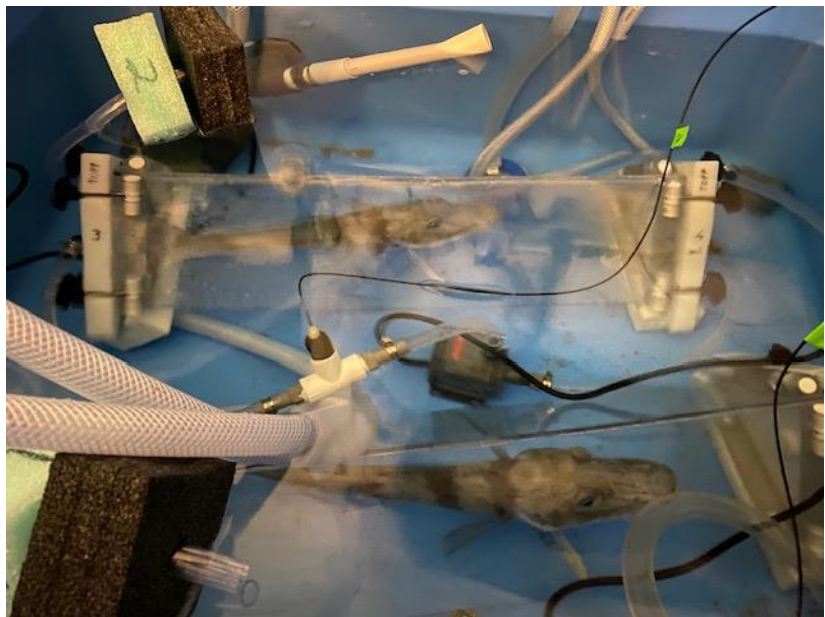
Chaenocephalus aceratus in respirometer tanks used to measure hypoxia tolerance. Image credit: Kristin O'Brien
